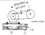
Tension new belts at the max. deflection force recommended for the belt section. Check the belt tension at least two times during the first 24 hours of operation. Any re-tensioning should fall between the min. and max. deflection force values.
